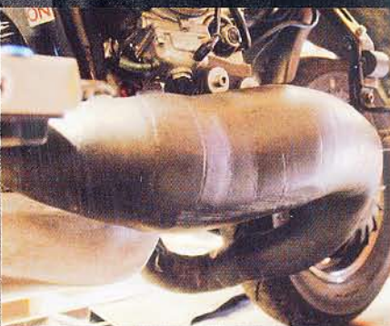
The main chamber actually sits where the flywheel cowling would have been.
