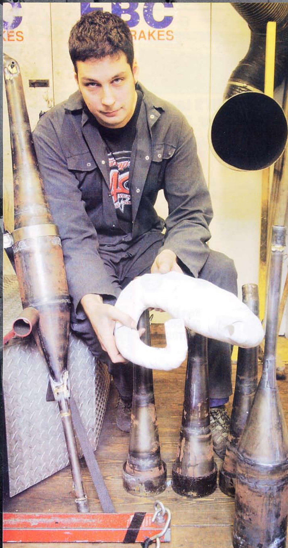
Charlie with just a few of the adjustable exhaust sections used to develop his race exhaust.
