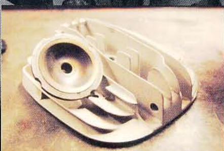
A blank Yamaha 400 head and one of the interchangeable combustion chamber domes.
