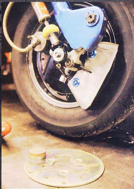
The EBC disc and pads that Charlie modifies for his front brake.
