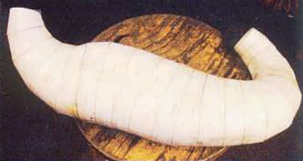
All the sections of the exhaust are designed in computer software. Charlie first makes the pipe in paper – then in cardboard – while trying to formulate a layout.
