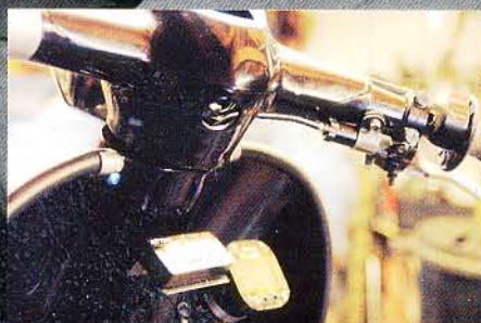
Thumb operated powerjet lever is used to add more fuel during a race when the motor starts to overheat.
